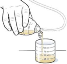
**5. Drain the fluid into a measuring cup.**
